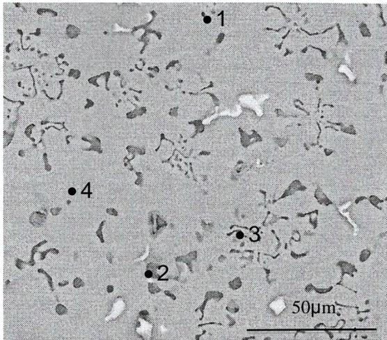
Figure 2. SEM examination on the composite with Al-9Zn-6Mg-3Si matrix with 5 % alumina reinforcement, dissolution temperature of 500 °C, holding time duration of 30 minutes, and aging temperature 200 °C .
