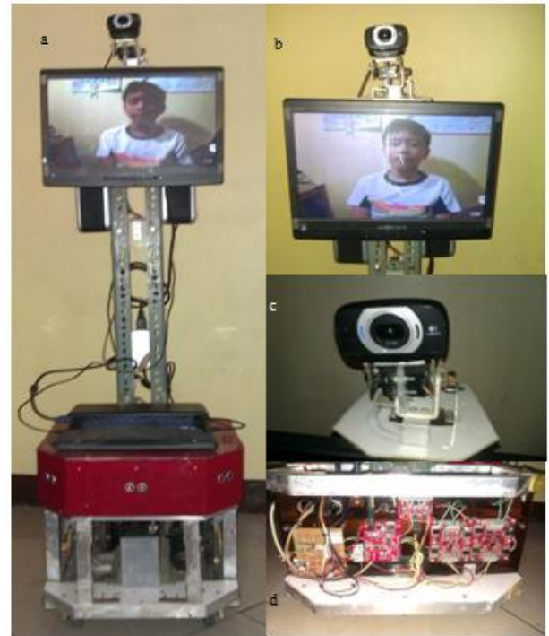
Figure 8. The overall robot system hardware: (a)overall robot system;(b)LCD video system and speakers;(c)Web camera mounted on pan and tilt servo mechanism; (d)Control electronics consisting of microcontrollers, motor controllers and power conditioning circuits.
