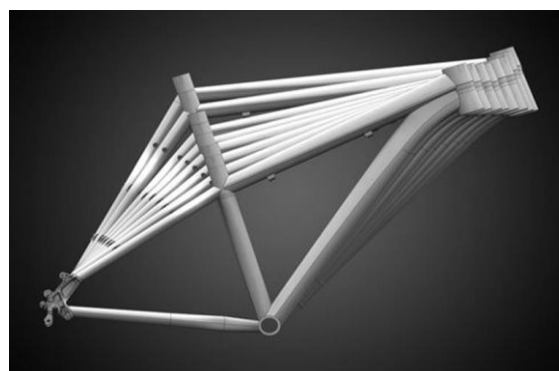
Figure 3 Scheme of differences in the size of the bike frame Mountain Bike
